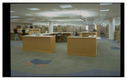
Illustration 8: Recessed fixtures with parabolic louvers provide lowglare lighting at the Sacramento Central Library.
