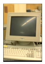
Illustration 12: Lights at service desks should be positioned so they do not reflect in computer monitors.
