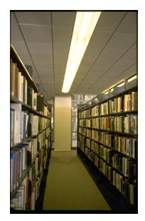
Illustration 4: Stack lighting runs parallel to the stacks at the San Francisco Main Library, and the lighting is very even from top to bottom of each stack.
