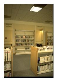
Illustration 10: Although recessed 2'x2' fixtures with parabolic louvers can provide low-glare lighting for reading tables, they do not light the perimeter of the space very well.
